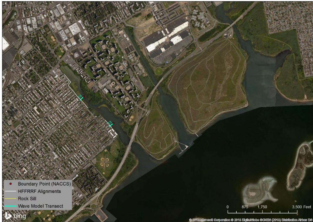
Figure D-2: 1-D wave model transect locations for refinement of Design Wave condition
