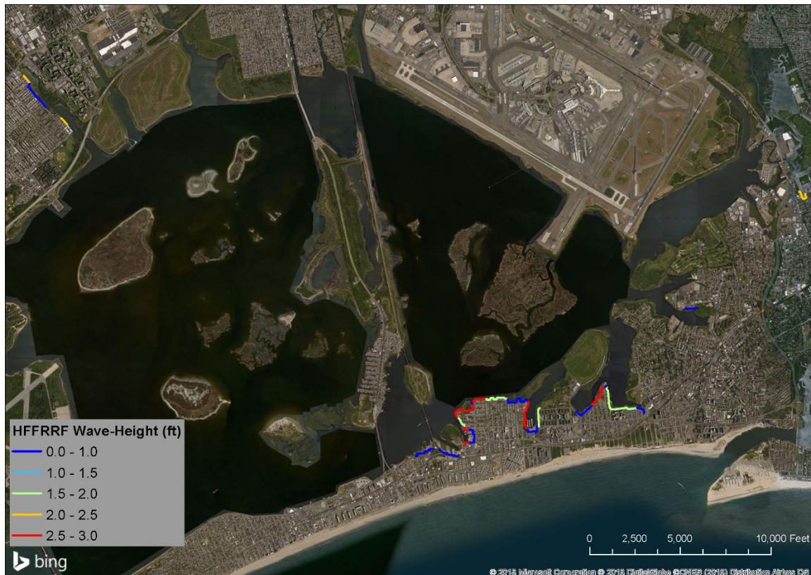
Figure D-8: Updated wave-heights at HFFRRF alignments using 1-D wave model to transform NACCS data
