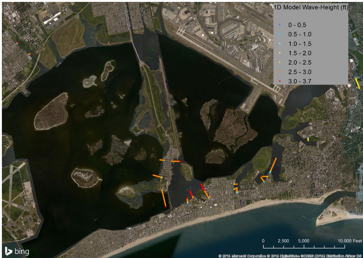
Figure D-3: Overview of wave model output showing predicted wave-heights
